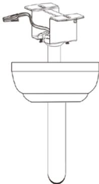
Insert the semi-spherical end of the rod into the bracket through the space provided: align the notch on the bracket with the corresponding slot in the semi-spherical end, and check that the electrical wires (both of the rod and of the mounting bracket) are positioned so as not to obstruct operation.
