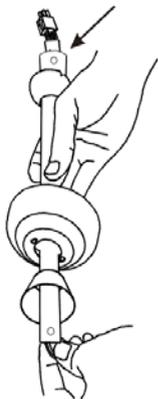
Thread the rod support (if previously removed or not present) so that it is positioned on the top flap (end three holes), then the top cap (2) and bottom cap (4); insert the electrical leads through the rod cavity. The wires should be inserted from the bottom upwards. Make sure no wires are on the outside.
