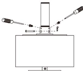
Insert the rod (the rod holder must be at the top) onto the motor body at the upper end, so that the holes are coaxial, and insert the appropriate pin, then secure it using the cotter pin (which must be inserted in such a way as to prevent both pin and cotter pin from slipping out). Then lock the rod by tightening the two safety screws.
