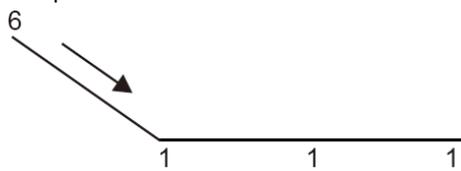
To activate the "Sleep" mode, press the button on the "
