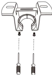
Loosen the two screws securing the top cap.
