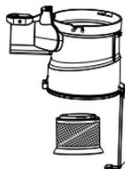
c) Rinse the filter under running water and dry it in the sunlight.
